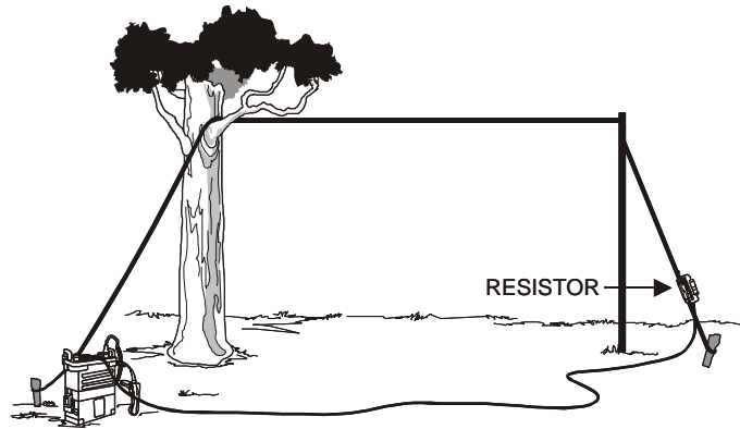
Figure 6-11. Long Wire Antenna.
