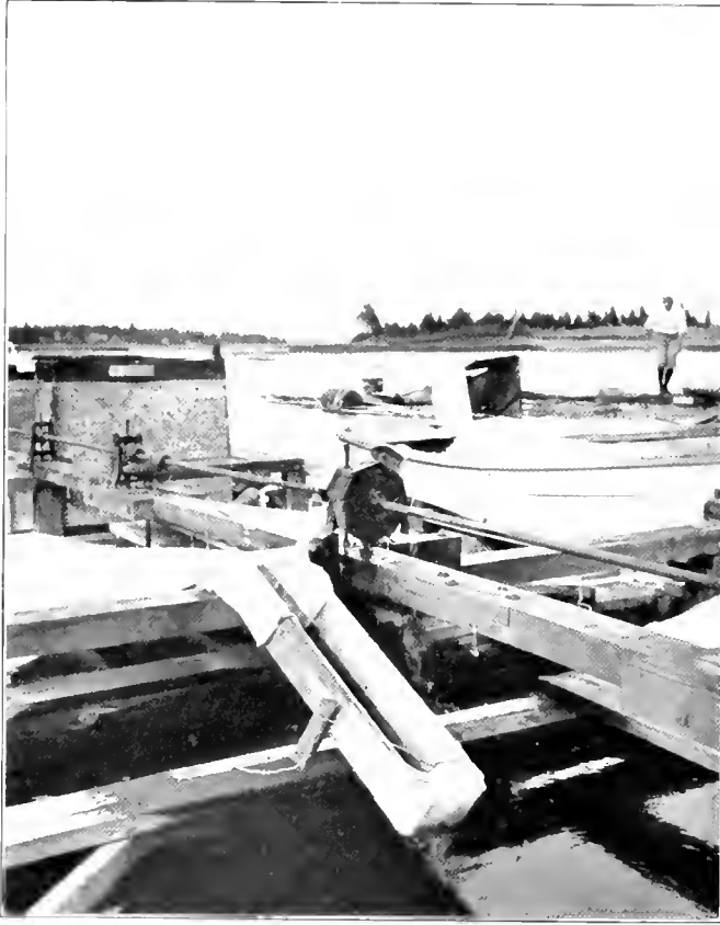
FIG. 15.—Filter car, same as figure 14, plate xcvi, showing bucket chain in operation. One of the buckets has just emptied itself and the stream of water is faintly shown running into the trough.
