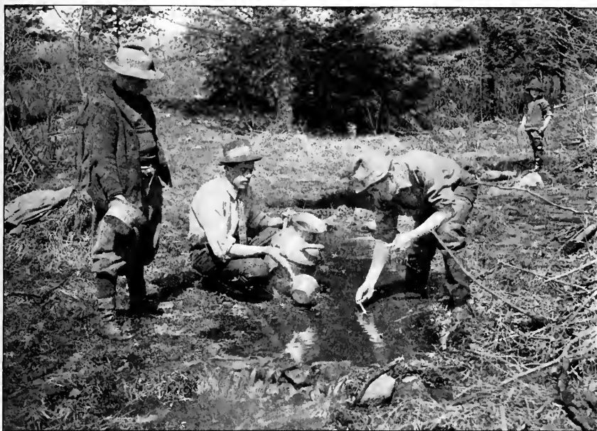
A dairy thermometer will give an accurate check on the temperature of the water in stream and can.
