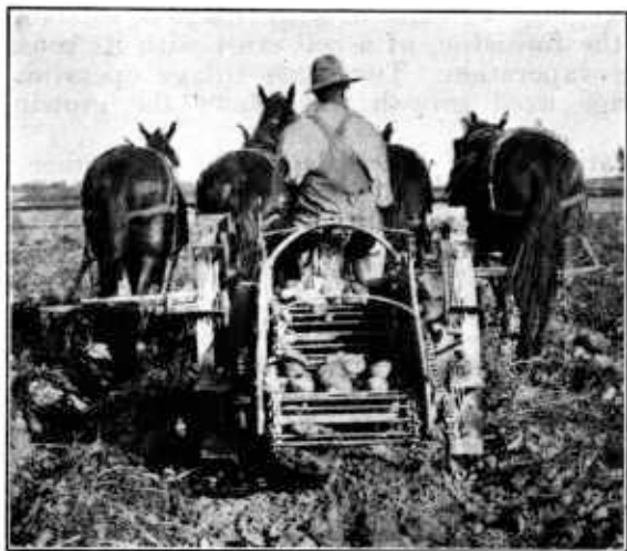
FIGURE 6.—Operating an elevator type of digger with four horses. Note the cloddy compact soil. (Near Greeley, Colo.)
