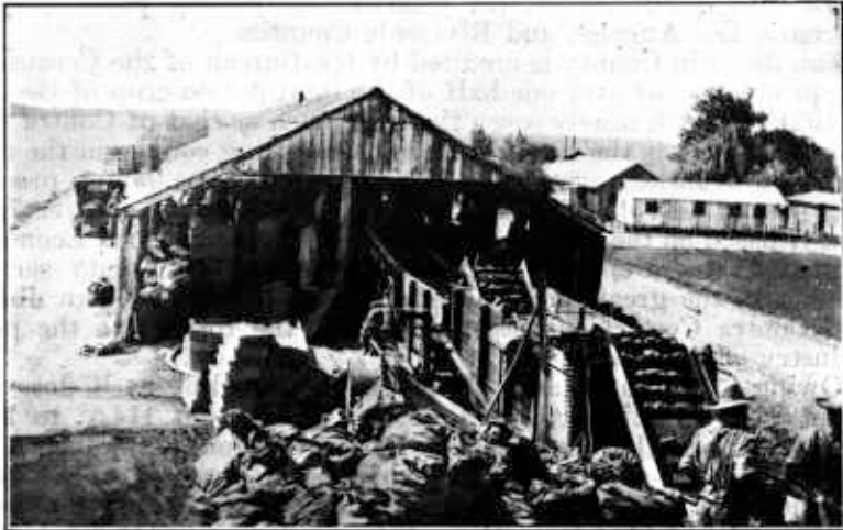
FIGURE 8.—Washing potatoes on the wholesale plan. The tubers come out of this washer well cleaned. They drop from the conveyor belt into huriap sacks, thus avoiding hand labor
