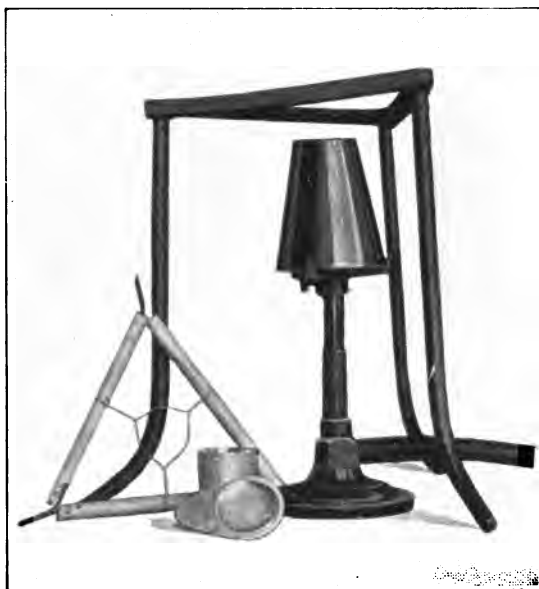
FIG. 8.—PLATINUM CRUCIBLE AND SUPPORT FOR COKE TEST.
