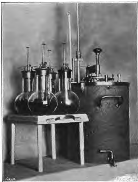
FIG. 21.—BOMB IMMERSSED AND READY FOR IGNITION OF THE FUEL.
