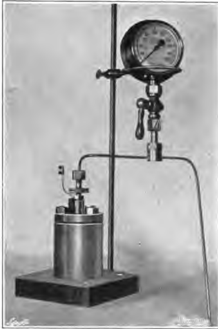
FIG. 19.—BOMB WITH OXYGEN SUPPLY CONNECTIONS AND PRESSURE-GAUGE.
