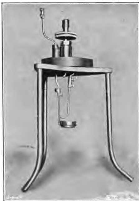
FIG. 18.—BOMB COVER WITH PLATINUM DISH AND IGNITION WIRE.
