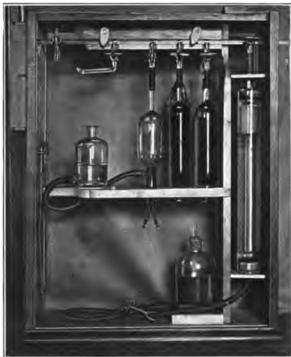
FIG. 37.—IMPROVED FORM OF ORSAT'S GAS-TESTING APPARATUS.
