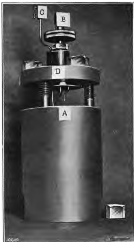
FIG. 16.—MAHLER-DONKIN BOMB CALORIMETER.
