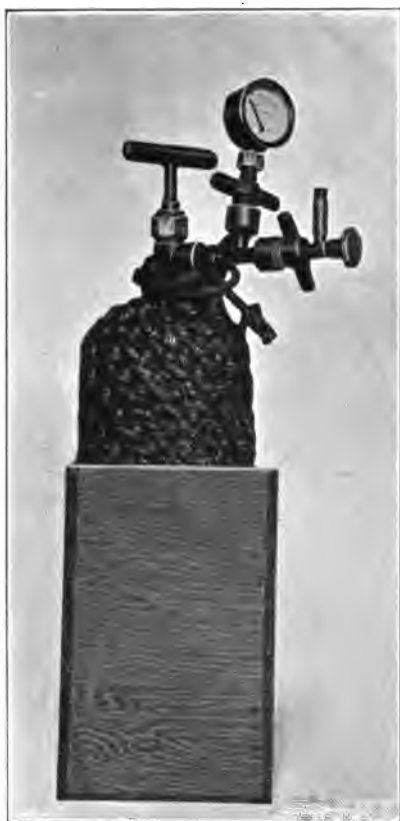
FIG. 20.—OXYGEN CYLINDER WITH REDUCING VALVE AND PRESSURE GAUGE.
