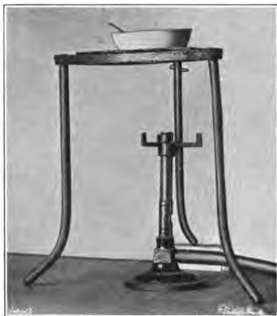
FIG. 7.—ARRANGEMENT OF APPARATUS FOR ASH TEST.
