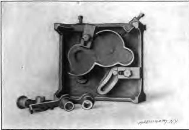
Fig. 1. Typical Open Drill Jig for Gear Guard
