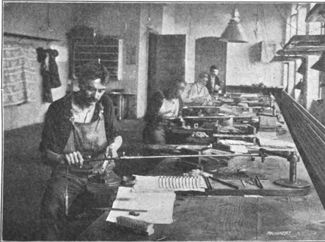
Fig. 34. Etching the Teeth in Files
