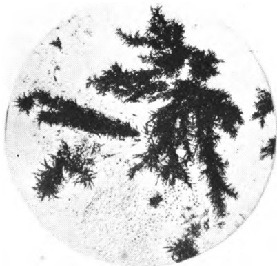
FIG. 6.—Tropacocaine 1 : 500. Crystals formed with zinc-chlor-iodide ( \times 150 ).
