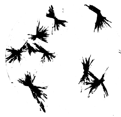
FIG. 6.—Morphine 1 : 50. Crystals formed with mercuric chloride (X150).
