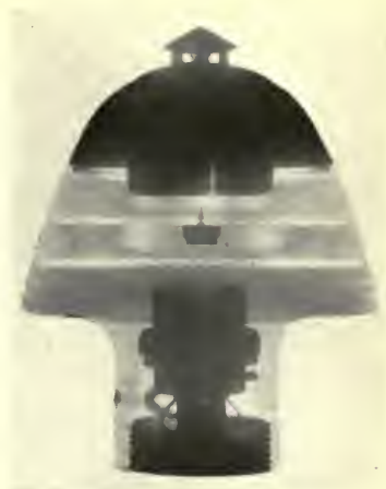
FIG. 62.—(A) Ordinary photograph of a Russian fuse. (B) Radiograph showing internal details (Pullin).
