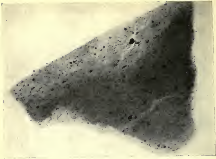
FIG. 89.—Radiograph of a block of carbon from the electrode of an electric arc furnace, showing mineral impurities (Pullin).
