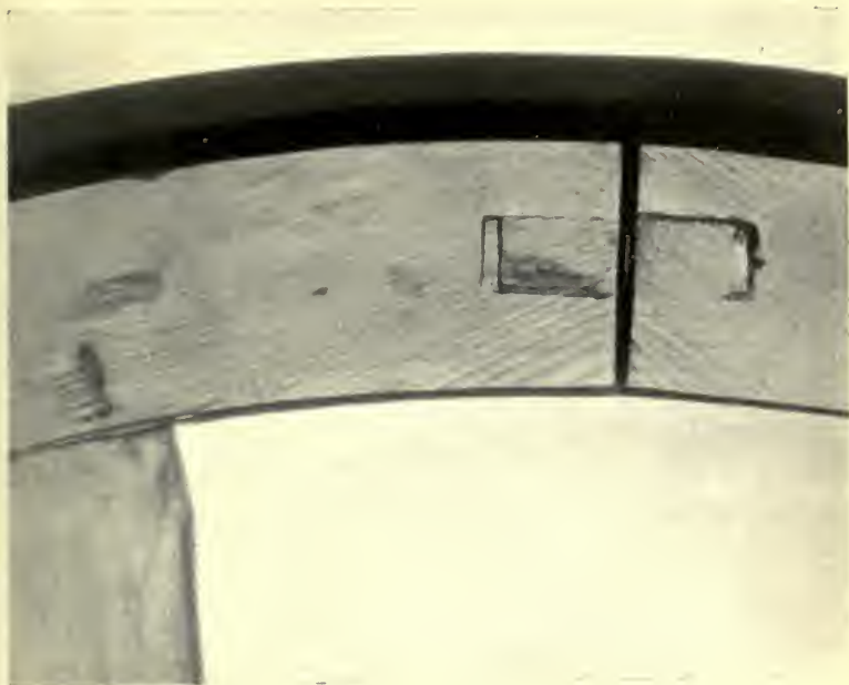
FIG. 78.—Radiograph of felloe of limber wheel, showing joint filled with lead paint (Pullin).
