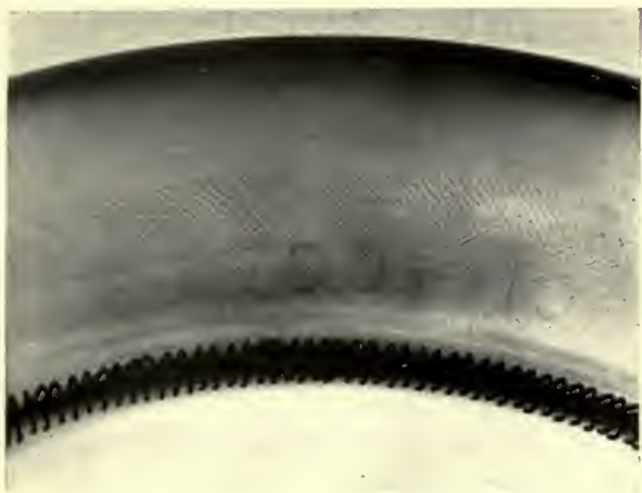
FIG. 79.—Radiograph of aeroplane tyre, showing corded structure under rubber (Knox and Kaye).
