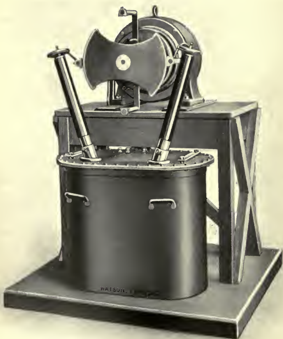
FIG. 18.—Oil-immersed transformer, with rotary converter and mechanical rectifier.
