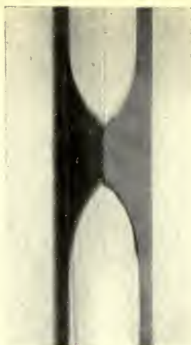
FIG. 74.—Radiograph of hollow wooden longeron of aeroplane, showing the registering of the internal stiffening blocks (Knox and Kaye).
