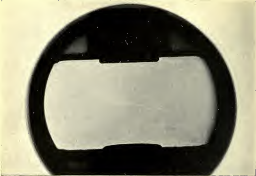
FIG. 68.—Radiograph of aluminium piston of aeroplane engine, showing crack.
