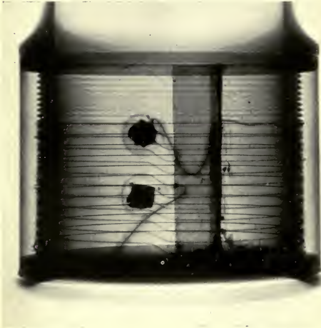
FIG. 83.—Radiograph of electrically heated porcelain coffee pot, showing concealed heating element.
