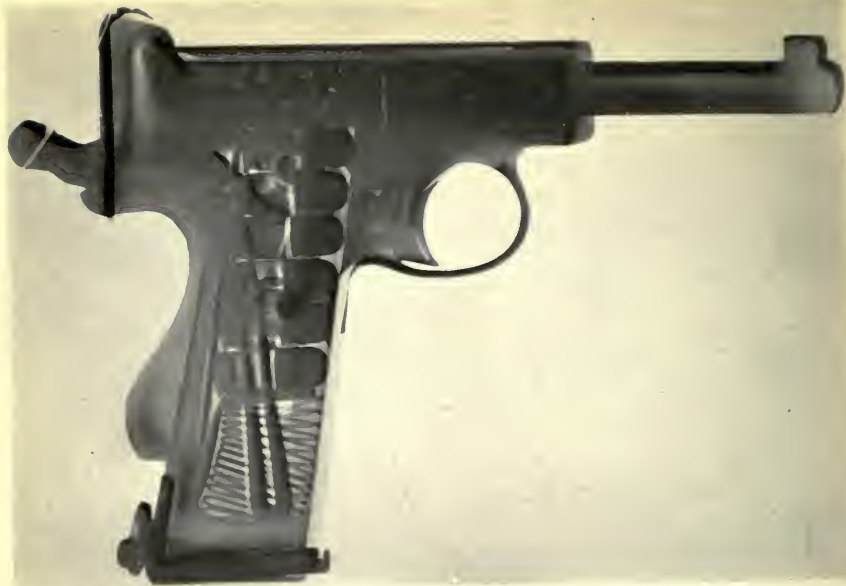
FIG. 64.—Radiograph of an automatic pistol, showing cartridges in chamber (Pullin).
