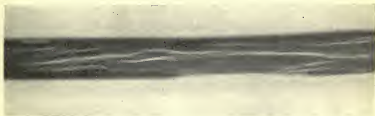
FIG. 88.—Radiograph of artificial graphite, showing internal cracks.
