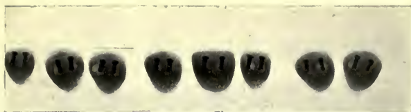
FIG. 86.—Radiograph of artificial teeth, showing gas bubbles present as a defect (Owen).
