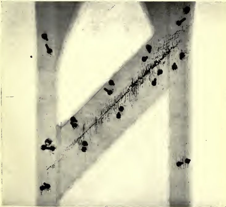
FIG. 71.—Radiograph of aeroplane hollow spar, showing concealed and prohibited joint in plywood sides (Knox and Kaye).
