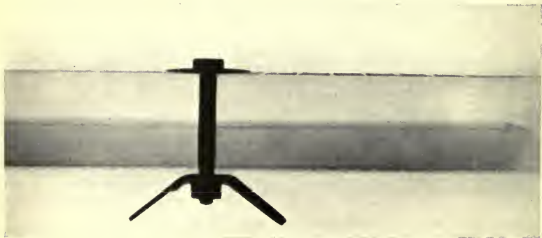
FIG. 77.—Radiograph showing nature of hidden splice in aeroplane spar (Knox and Kaye).
