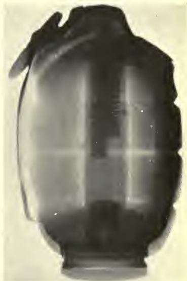
FIG. 63.—(A) Ordinary photograph of hand grenade. (B) Radiograph showing detonator and also flaws in the metal (Pullin).
