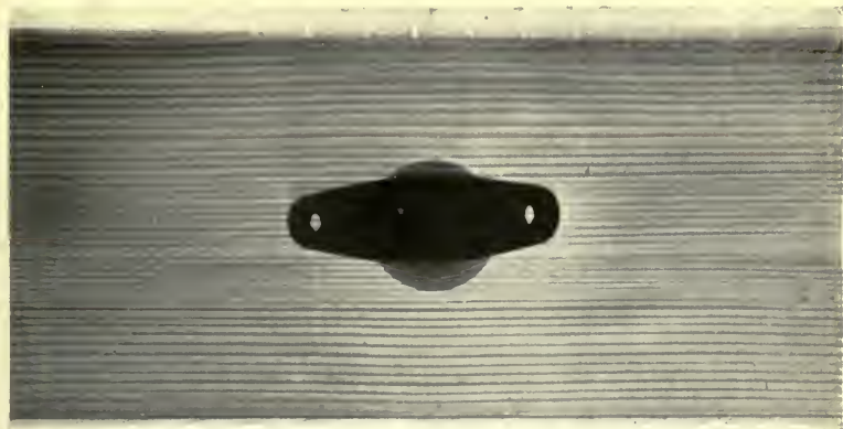
FIG. 66.—Radiograph of perfect specimen of silver (sitka) spruce aeroplane spar, showing annual rings. Also aluminium washer and steel wiring plate (Knox and Kaye).
