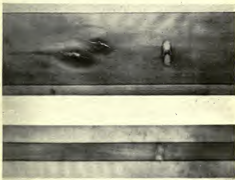
FIG. 75.—Radiograph (front and side view) of laminated wooden aeroplane spar, showing in centre lamina forbidden knots and grub hole which were quite concealed from view (Knox and Kaye).
