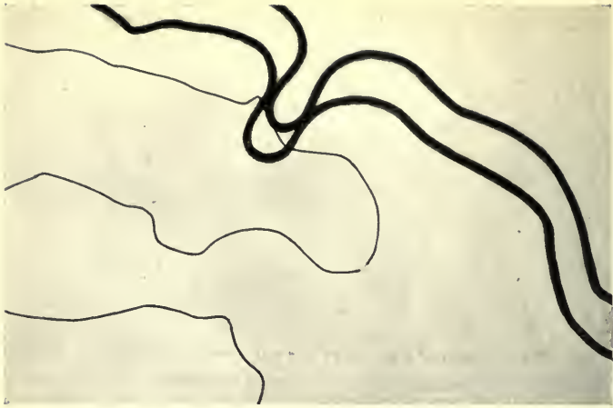
FIG. 84.—Radiograph of aeroplane pilot's electrically heated leather jacket, showing break in heating element. These jackets are indispensable to pilots flying at very high altitudes.
