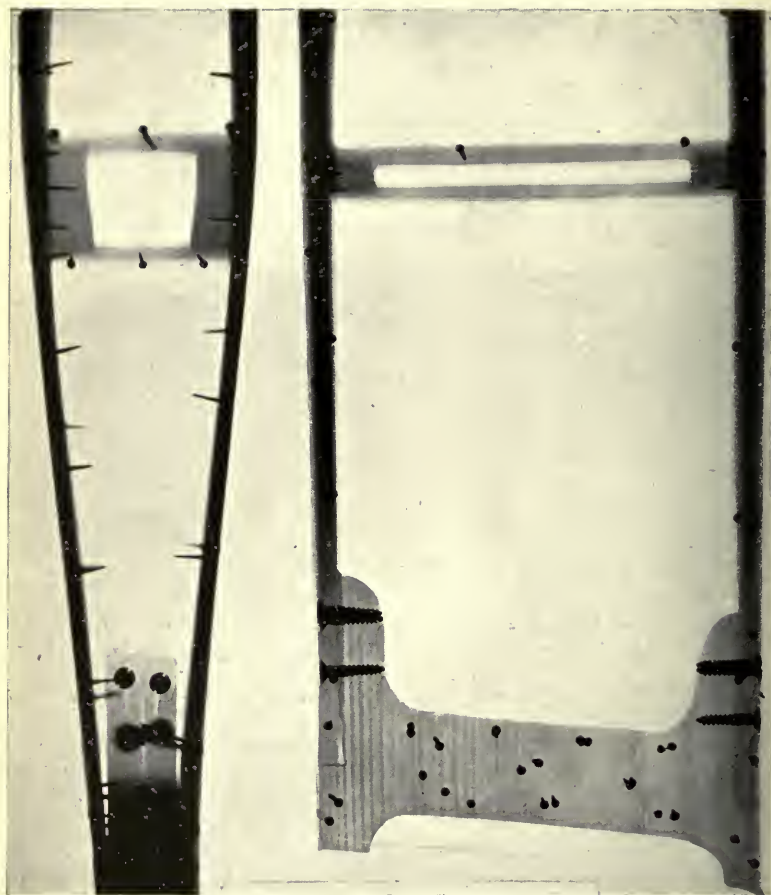
FIG. 72.—Radiograph (side and front views) of hollow aeroplane wooden spar, showing badly shaped end block split by screws. This was quite concealed from view (Knox and Kaye).
