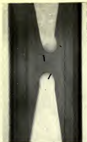
FIG. 73.—Radiograph of hollow main-wing aeroplane spar of wood. The internal strengthening block is split and shows poor workmanship (Knox and Kaye).
