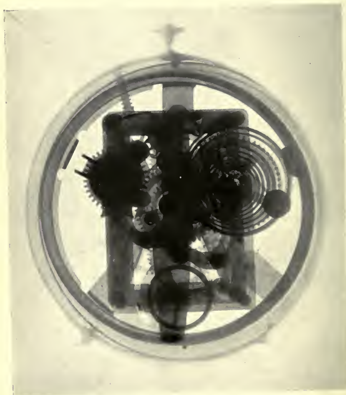
FIG. 65.—Radiograph of an alarm clock taken through the case (Thorne-Baker and Levy).
