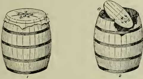
Barrel traps: 1, with stiff paper cover; 2, with hinged barrel cover; a , stop; b , baits. (After Biological Survey.)
