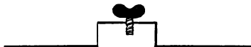
FIG. 198.—SHAPE OF SIDE IRONS HOLDING THE AXLE OF FAN IN "NO NAME'S" BLOWER.
