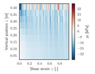
**Figure 11.** Temporal evolution (x axis) of horizontally averaged fluid pressures (y axis). The permeable material (top) is able to quickly respond to internal volumetric changes, which are shortlived and of small magnitude. The low-permeability material (bottom) is dominated by large pressure reductions and relatively slow relaxation.
