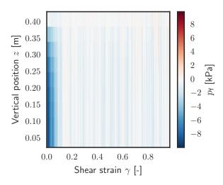
Relatively impermeable ( $k_c = 3.5 \times 10^{-15} \text{ m}^2$ )
