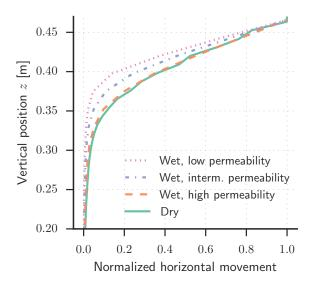
**Figure 8.** Horizontal particle displacement with depth (shear strain profiles) for the dry and fluid-saturated shear experiments. Top: displacement profiles from experiments with different shear velocities. Bottom: displacement profiles from experiments with different permeabilities.
