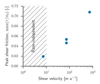
**Figure 6.** Peak frictional strength before the critical state of the low-permeability granular bed ( $k_c = 3.5 \times 10^{-15} \text{ m}^2$ ) at different shear velocities. The frictional strength is constant and rate independent at velocities lower than  $10^1 \text{ ma}^{-1}$  as pore-pressure diffusion rates far exceed rates in volumetric change.
