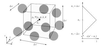
**Figure 2.** Left: a cell in the fluid grid. The node for pressure  $(p_f)$ , the gradient of fluid pressure  $(\nabla p_f)$ , porosity  $(\phi)$ , permeability (k), and average grain velocity  $(\overline{v})$  are calculated at the cell center. Right: the weight function (Eq. 6) at various distances.
