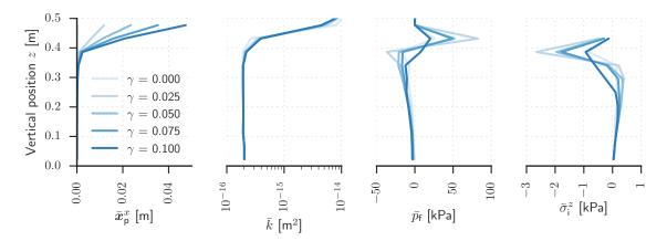
Figure 10. Horizontally averaged fluid and particle behavior with progressive shear strain. (left) Vertical particle displacement, (center left) mean permeability, (center right) mean fluid pressure, and (right) vertical component of the mean fluid stress, calculated as  $f_i^i/A^i$ , where  $f_i^i$  is the fluid pressure force on particle i from Eq. (12) and  $A^i$  is its surface area. Note that the limits of the horizontal axes differ between the experiments.
