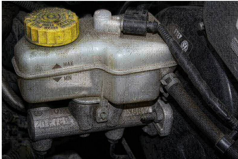
A brake fluid reservoir. Notice the MAX and MIN markings. Image credit: CC-BY-Frettie on Wikipedia
