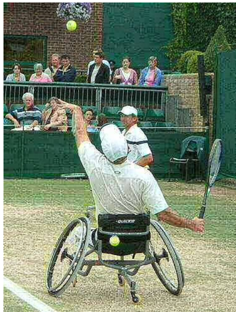
A wheelchair with an inward camber as seen on many athletic wheelchairs.
