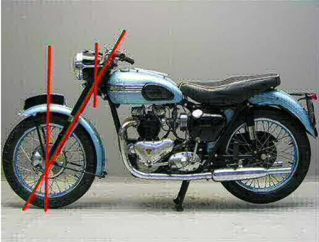
A positive caster is easily seen on the front wheels of motorcycles and bicycles. Image adapted, original credit: CC-BY-SA-Yesterdays Antique Motorcycles on Wikipedia
