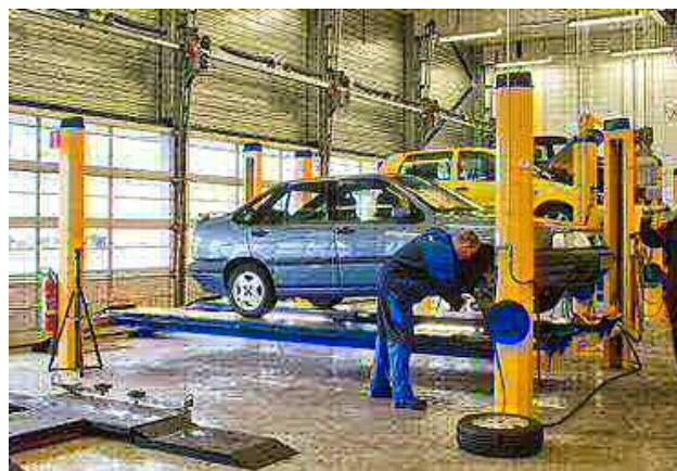
Another hydraulic lift that raises the car on its tires
