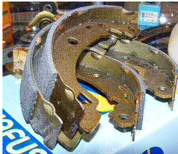
Drum brake shoes (violet color) and linings.
