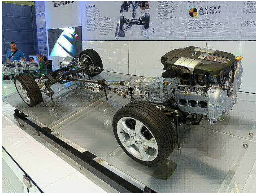
Powertrain for a Subaru vehicle. The engine and transmission are seen on the right. The drive shaft is in the middle and the differential is on the left at the center of the rear axle.
