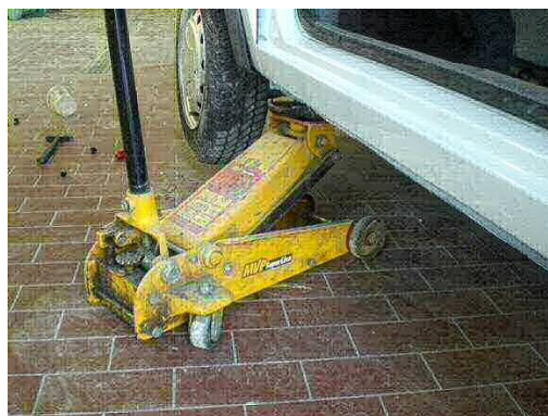
Hydraulic jack with hand-pump mechanism
