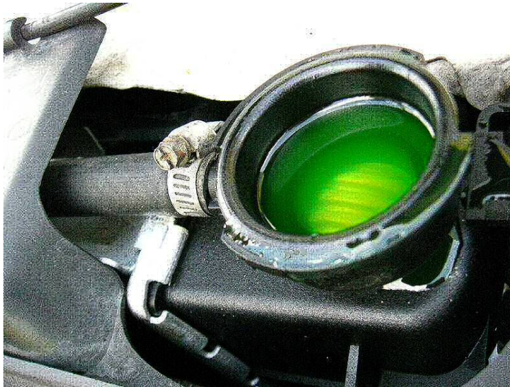
Coolant. Notice the green color; coolant can actually be any color (pink, orange, transparent, red, etc.) Image credit: CC-BY-EvelynGiggles on Wikipedia
