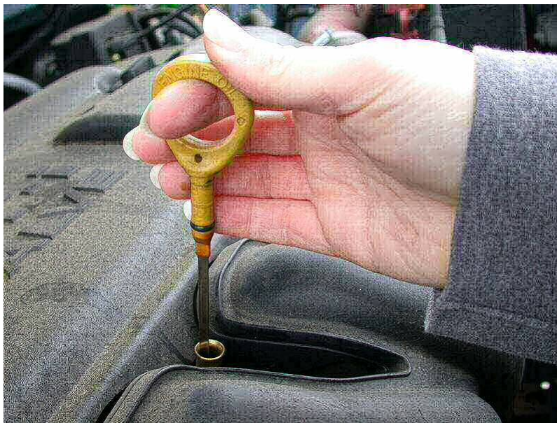
Oil dipstick (above) and oil level on a dipstick (below) Image credits: both CC-BY-SA-Dvortygirl on Wikipedia
