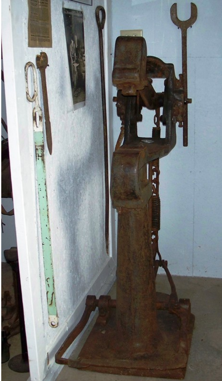
Treadle Hammer in place in the blacksmith shop, Sterling
