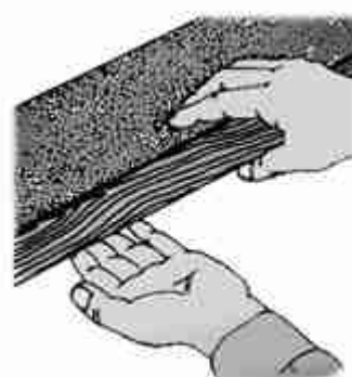
FIG. 16 - Edge stripping should be slightly wider than the edge to be covered. The extra width goes at the bottom.
