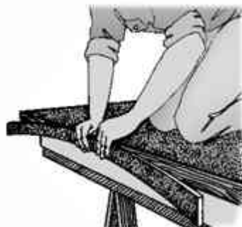
FIG. 13 - After applying two coats of cement to edges, apply one coat to back of laminate.
