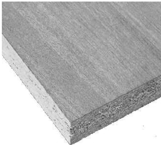
Particle board is sandwiched between laminates
