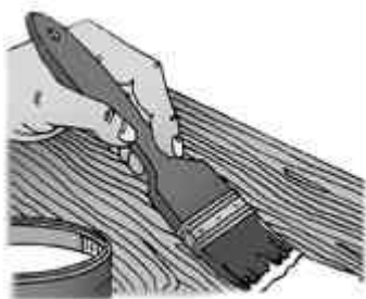
FIG. 5 - Brush contact cement over the counter surface after sanding and cleaning it.
