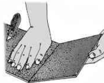
FIG. 4 - The laminate will snap after it is scored
