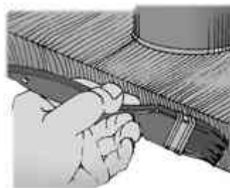
FIG. 6 - Apply two or three coats of contact cement on any trim strips along the vertical edges.
