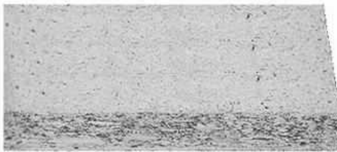
Flaky texture is visible at the cut edge
