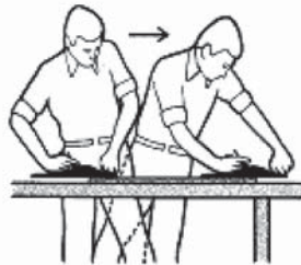
How to plane end grain
