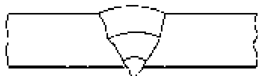
Excess Weld Metal at the Root
