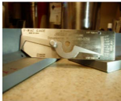
Figure 17: Bridge cam gauge
