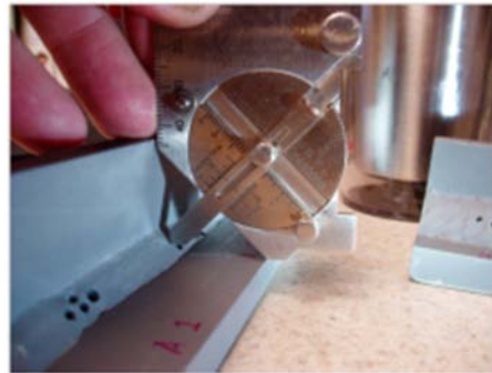
Figure 16: Throat measurement with cam gauge
