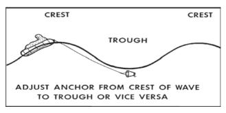
Figure II-11. Sea Anchor Deployment
