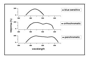
Figure 3 - Spectral response curves for three types of film with different spectral sensitivities (after [7])
