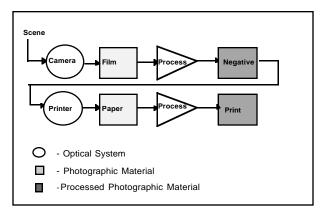
Figure 1 - Block diagram of the print photography process
