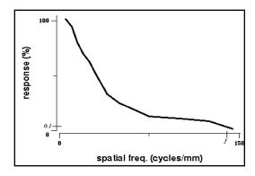
Figure 4 - Modulation Transfer Function (MTF) of a typical emulsion (after [15]).
