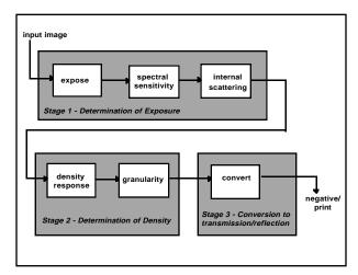
Figure 5 - Simulation pipeline for a single processing step
