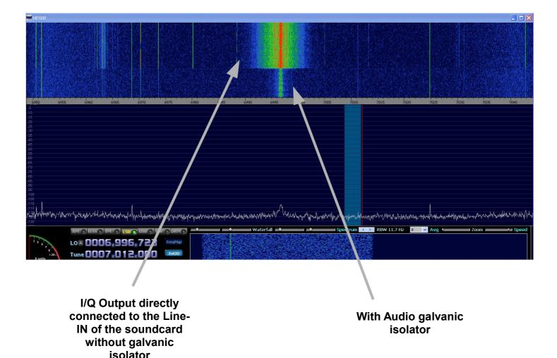
The follow example show the spectrum with a built-in RealtekHD at 48kHz samplingrate on a PMSDR:
