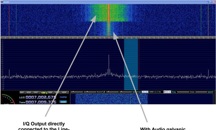
I/Q Output directly connected to the Line-IN of the soundcard without galvanic isolator
