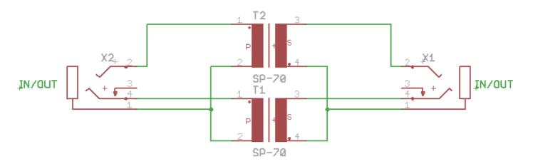
The audio galvanic isolator is build by a couple of broadband audio transformers and have a symmetrical design. The input / output impedance is 600 Ohm (turn ratio = 1:1), therefore you can also invert the input and output connections.
