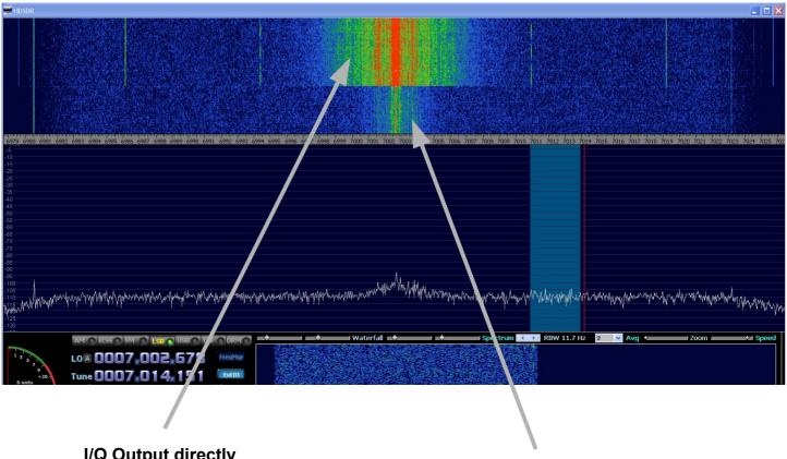
I/Q Output directly connected to the Line-IN of the soundcard without galvanic isolator
