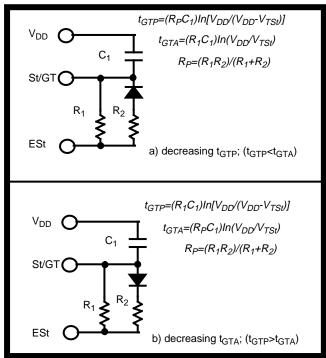
Figure 5 - Guard Time Adjustment
