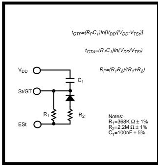
Figure 8 - Non-Symmetric Guard Time Circuit
