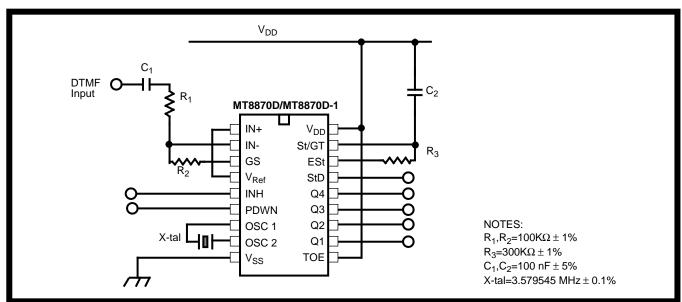
Figure 10 - Single-Ended Input Configuration
