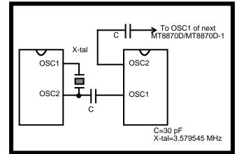
Figure 7 - Oscillator Connection
