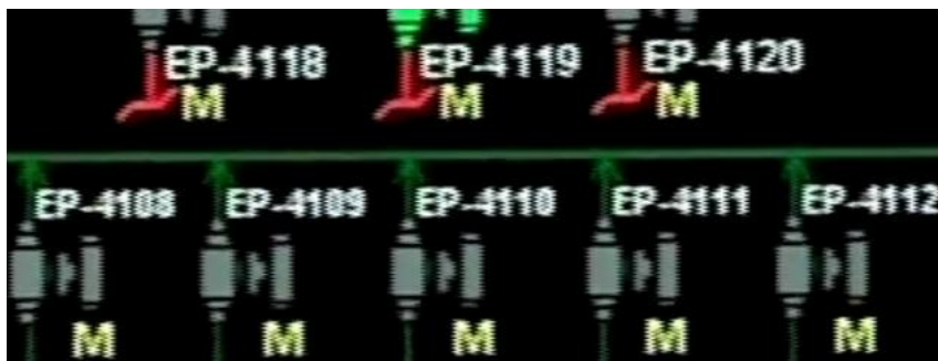
Figure 8: Very different valves: While the stage exhaust valves (labeled EP-4108 to 4112 in this partial screenshot from the CPS SCADA display) stay closed during normal operation and during the attack , at least one of the feed valves (labeled EP-4118 to EP-4120) must stay open. Pressure controllers at the product and tails take-offs must also be compromised to not signal a low pressure condition.
