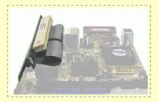
This will place the network card directly above the mainboard, and the whole assembly will
