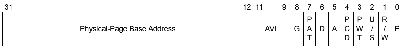
Figure 5-6. 4-Kbyte PTE—Non-PAE Paging Legacy-Mode
