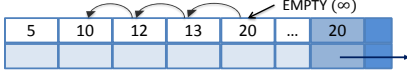
Figure 7. Deleting key 10 from a chunk. All keys greater than 10 are moved one entry to the left.
