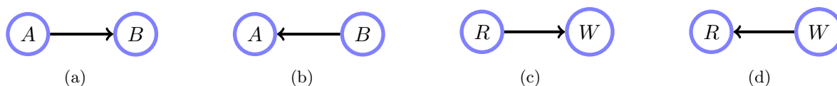
Figure 3.12: Both (a) and (b) represent the same distribution p(a, b) = p(a|b)p(b) = p(b|a)p(a) . (c): The graph represents p(\text{rain}, \text{grasswet}) = p(\text{grasswet}|\text{rain})p(\text{rain}) . (d): We could equally have written p(\text{rain}|\text{grasswet})p(\text{grasswet}) , although this appears to be causally non-sensical.
