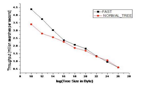
Figure 1. Throughput (million searches per second) of Normal Tree and Fast Tree
