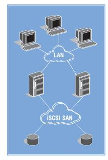
iSCSI is a proposed industry-standard that allows SCSI I/O commands to be sent over a network using the popular TCP/I P protocol. This is analogous to the way SCSI commands are already mapped to Fibre Channel, parallel SCSI, and SSA media. The proposal was made to the IETF (Internet Engineering Task Force) standards body jointly by Cisco Systems, Inc. and IBM.
