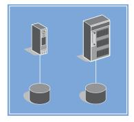
Direct Attached Storage is storage that is generally restricted to access by a single host (processor); sometimes by two hosts in small cluster (failover or failback) configurations. Even an enterprise-class disk system such as an IBM Enterprise Storage Server<sup>™</sup> (ESS) can be effectively configured as DAS by assigning portions (partitions) of the internal disk capacity to
