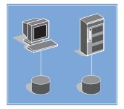
Direct attach—a single storage device is connected to a single processor (host).
