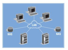
NAS: Network Attac hed Storage. A NAS device ("appliance"), usually an integrated processor plus disk storage, is attached to a TCP/I P-based network (LAN or WAN), and accessed using specialized file access/file sharing protocols. File requests
