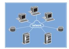
Network attach—one or more processors are connected to one or more storage devices.
