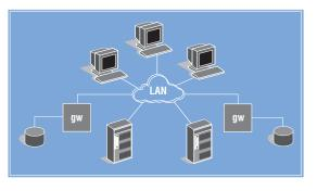
A NAS gateway provides the function of a conventional NAS appliance but without integrated disk storage. The disk storage is attached externally to the gateway, possibly sold separately, and may
