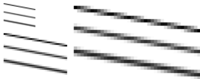
Figure 7.3: The results of the Wu, GS and optPoly algorithms at 1x, 2x and 4x magnification with nearest-neighbor resampling.
