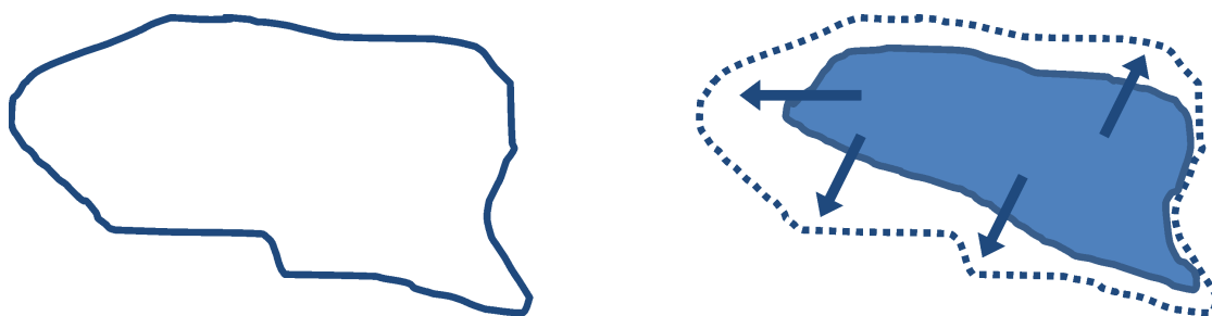
Figure 6.1: A region is obtained by expanding an initial candidate formed from homogeneous pixels.
