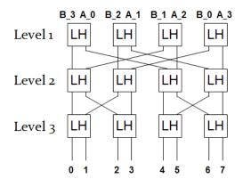
Figure 2: Bitonic merge network for merging sequences of length 4 elements each.
