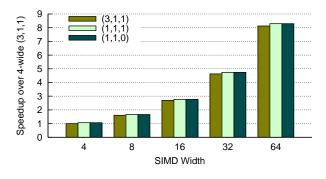
Figure 9: Speedup as SIMD width increases from 4-wide to 64-wide for different latencies of (a, b, c).
