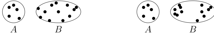
Figure 8.9: Illustration of the objection to the consistency axiom. Reducing distances between points in a cluster may suggest that the cluster be split into two.
