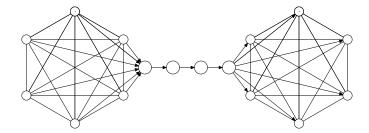
Figure 2: Two k-cliques joined by a unidirectional path of  $\ell$  nodes: terminating even one step earlier than stabilisation completely miscalculates the distance cdf (see Figure 1); the effective diameter is  $\ell+1$ , but terminating even just one step earlier than stabilisation yields an estimated effective diameter of 1.
