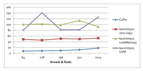
FIGURE 2: API OVERHEAD + GPU MEMORY I/O, 1 BLOCK, MAXIMUM (VECTOR INCREMENT)
