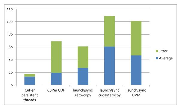
FIGURE 6: 1K VECTOR SUM + API OVERHEAD + GPU MEMORY I/O
