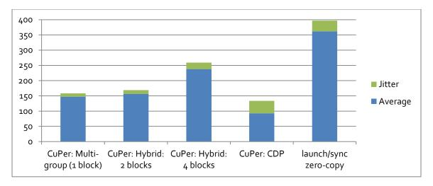
FIGURE 9: 128X128 MATRIX MULTIPLICATION + API OVERHEAD + GPU MEMORY I/O
