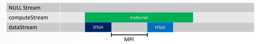
With a GPU-aware MPI stack, the Host<->Device traffic can be omitted:
