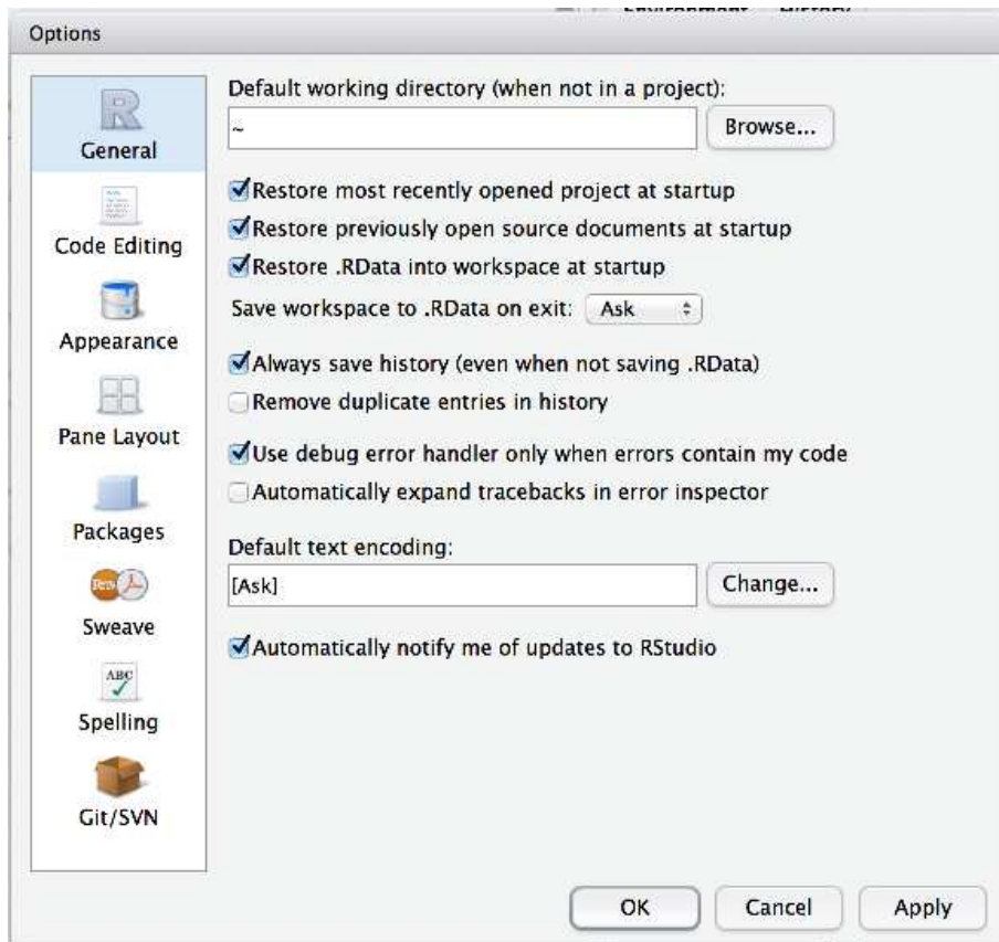
Figure 3.6: The options window in Rstudio. On a Mac, you can open this window by going to the “Rstudio” menu and selecting “Preferences”. On a Windows machine you go to the “Tools” menu and select “Global Options”.
