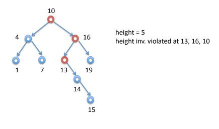
All is well at the node labeled 14: the left subtree has height 0 while the right subtree has height 1. However, at the node labeled 13, the left subtree has height 0, while the right subtree has height 2, violating our invariant. Moreover, at the node with key 16, the left subtree has height 3 while the right subtree has height 1, also a difference of 2 and therefore an invariant violation.
