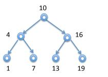
height = 3 height inv. satisfied If we insert a new element with a key of 14, the insertion algorithm for binary search trees without rebalancing will put it to the right of 13.
