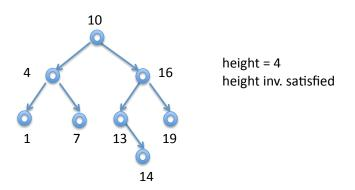
Now the tree has height 4, and one path is longer than the others. However, it is easy to check that at each node, the height of the left and right subtrees still differ only by one. For example, at the node with key 16, the left subtree has height 2 and the right subtree has height 1, which still obeys our height invariant.
