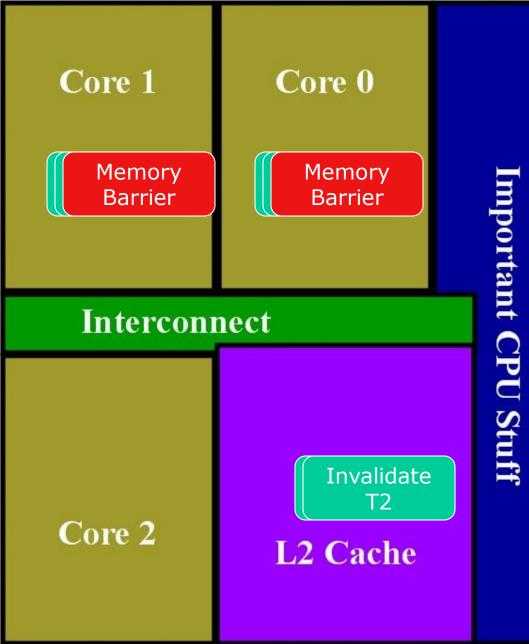
Proc 1: Write T1 MemoryBarrier(); Read T2 Proc 2: Write T2 MemoryBarrier(); Read T1
