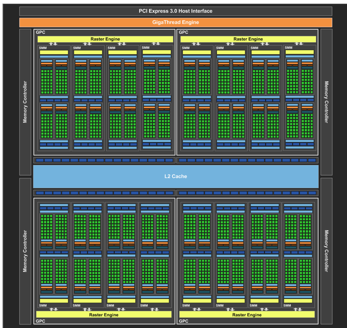
Figure 2: GM204 Full-chip block diagram
