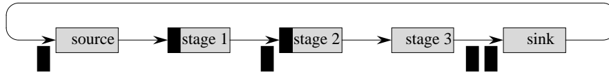
Figure 2.1: A standard FG pipeline comprising a source, a sink, and three other stages. Each black rectangle represents a buffer. Where a buffer appears inside a stage, the stage is currently working on that buffer. Buffers in queues appear below the arrows between stages. The arrow from the sink to the source represents how buffers are recycled.
