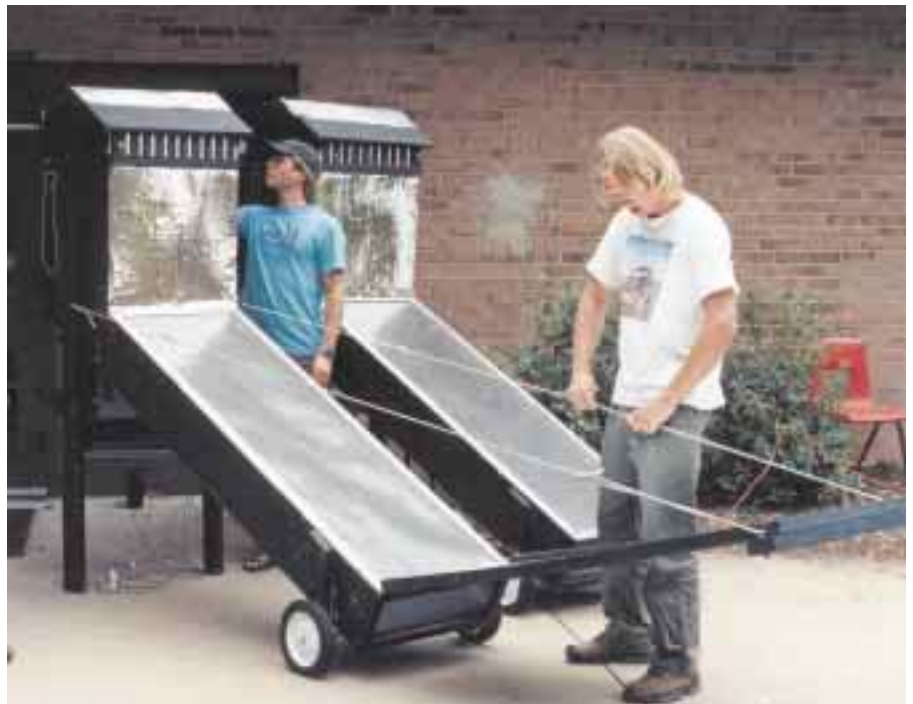
Above, Photo 4: Setting the front reflector angle.
