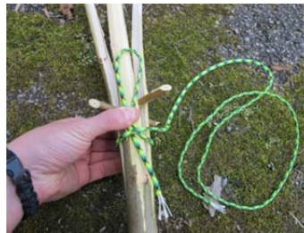
Wrap the long end around the gig and over the short end.
