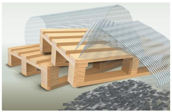
The Prepper Project blueprints show all the details for building an electricity-free "fridge" to keep foods at least 20°F cooler than surrounding air. Shipping pallets can be used to built the wooden framework, one pallet for each side of the fridge. The same metal lath that's ideal for a drum smoker charcoal basket makes a perfect screen to contain the charcoal that lines the walls. Look for lath in wrecked buildings or building supply yards.
