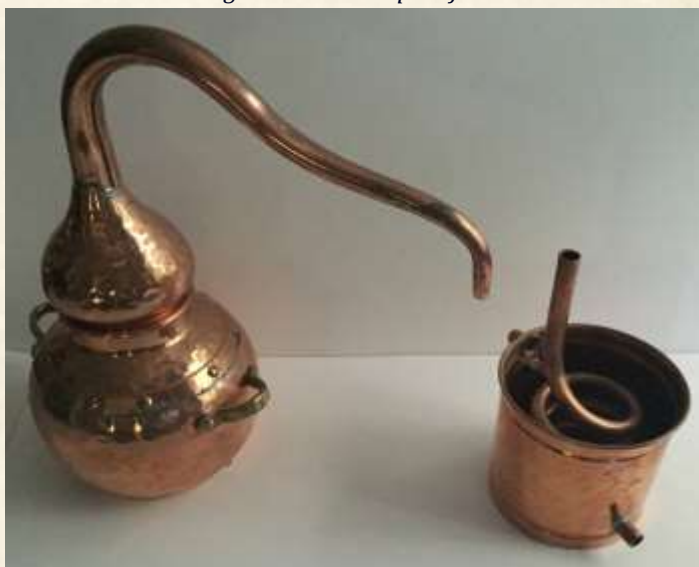
Alembic still showing column decoupled from the condenser:
