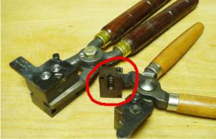
(Two bullet molds. The single cavity mold is open and empty. The double cavity mold is closed and contains two bullets – Photo Credits: Thewellman)
