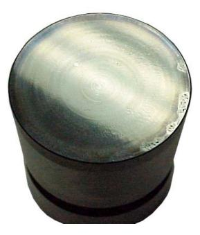
FIGURE 6 MINOR SPALLING
