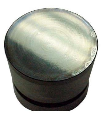
FIGURE 8 ACCEPTABLE LIFTER FACE SIGNATURE
