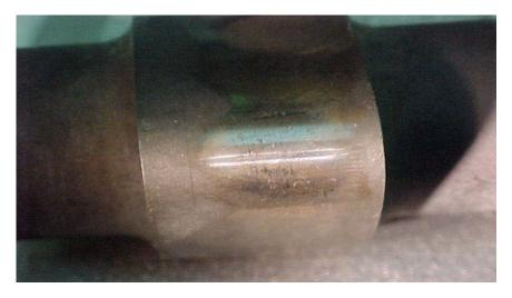
FIGURE 13 CAM LOBE APEX MINOR DISTRESS
