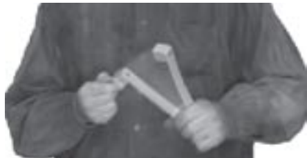
The bumping of a lock using the 'Tomahawk'.
