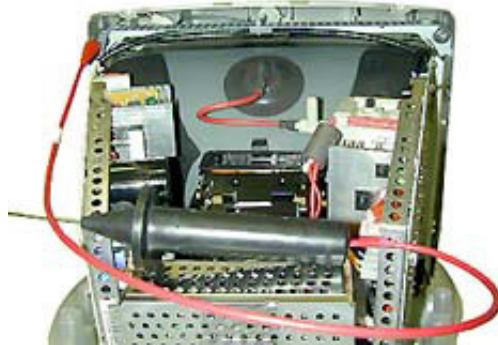
CRT Discharge Tool Connected to the Ground Lug
