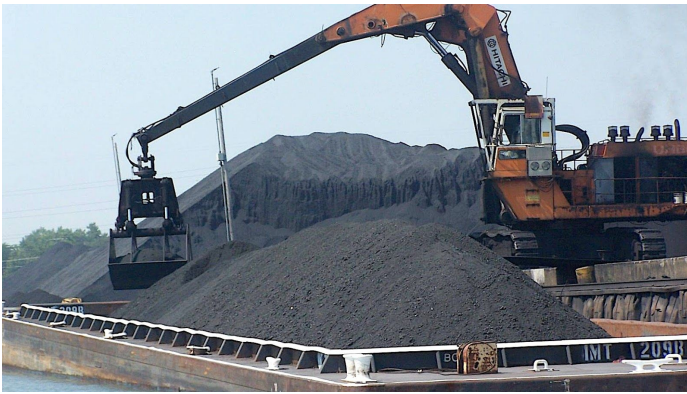
Filling barges with petcoke outside Chicago, Ill, USA (photo)
