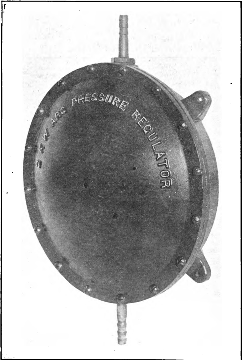
FIG. 14. Pressure regulator for use with Federal 2 Kw. Arc Converter Unit.
